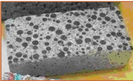
The use of wood and rubber can also be done together with other materials to produce elements such as bricks that will be used for the construction of interior partition walls. Small and large particles of both materials may in fact be used as reinforcing elements within a matrix of gypsum and/or cement, with a percentage weight varying from 25 to 50%.
